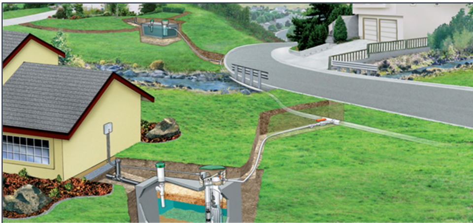
Septic Tank Effluent Pump (STEP) Collection System
