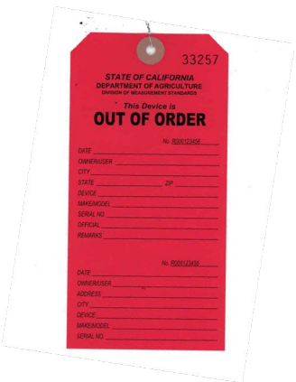
Figure 4 "Red Tags" are used to mark a device as out of service pending repair.
