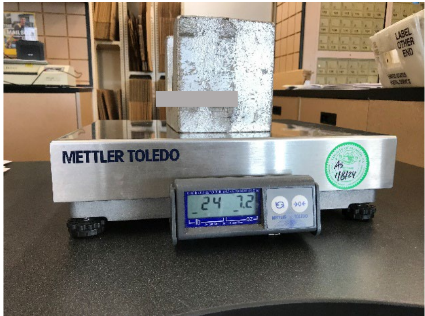
Figure 8 An example of a scale that failed a routine inspection. With 25 lbs. of known weight, the scale under-registered. This scale would be marked for repair, but the owner would be allowed to use it pending correction because the error is in the favor of the customer.
