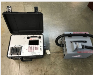
Figure 6 An electric vehicle charging station prover used to measure delivered quantities of electricity.
