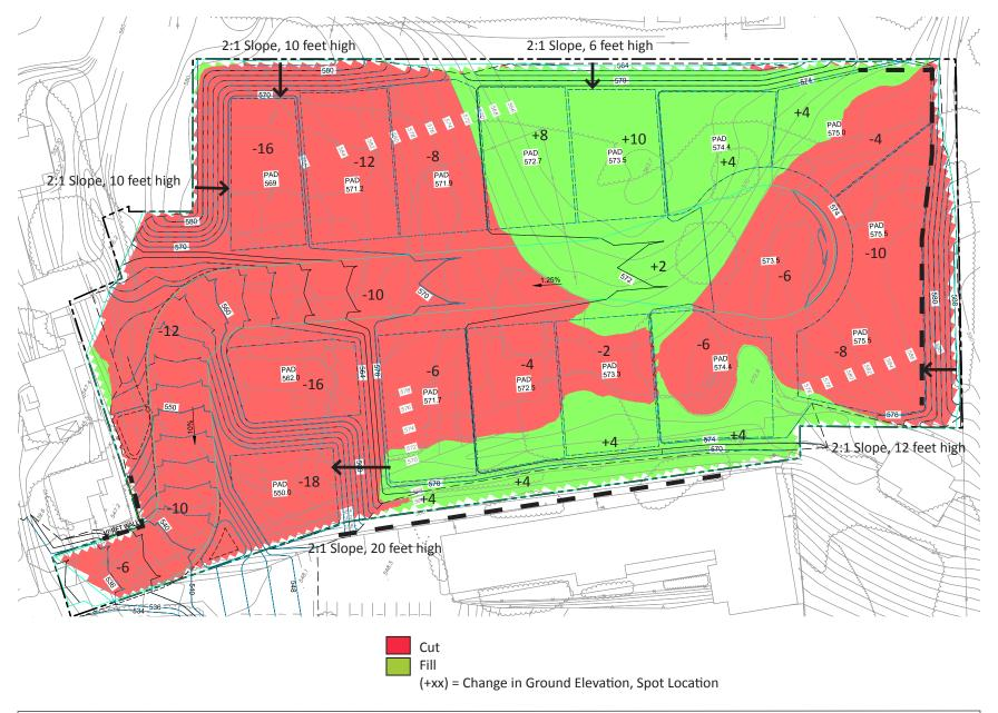
Figure 9-3 Cut and Fill Diagram, Tract 8297
